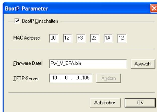
Figure 2-8 “BootP Parameters” (“Boot-Parameter”) dialog box in Factory Manager
